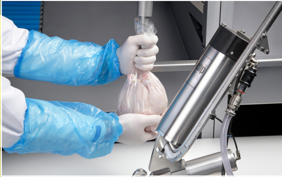
Vertical vacuum nozzle (pulling nozzle) in combination with the clipping machine EZ 600 of the Easy Clip Line®
