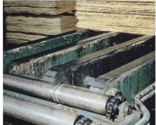
Straight Running: Steel and Stainless Steel Top Plates, 19.05 mm \triangleq 3/4" Pitch
