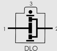
In-Line Series combines a high quality planetary differential with an irreversible worm gear in one housing, allowing infinite angular adjustment of the output shaft.
