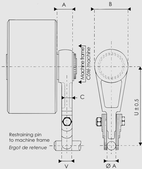
When fitted to the reaction sleeve, the torque arm holds the sleeve stationary.
