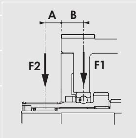
The design of the REDEX unit does not permit axial loads to be sustained.
