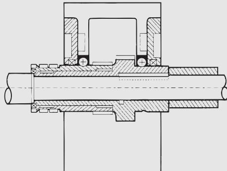
The accessory fitted to the reaction sleeve must be adjacent to the bearing to avoid excessive bending of the supporting shaft
