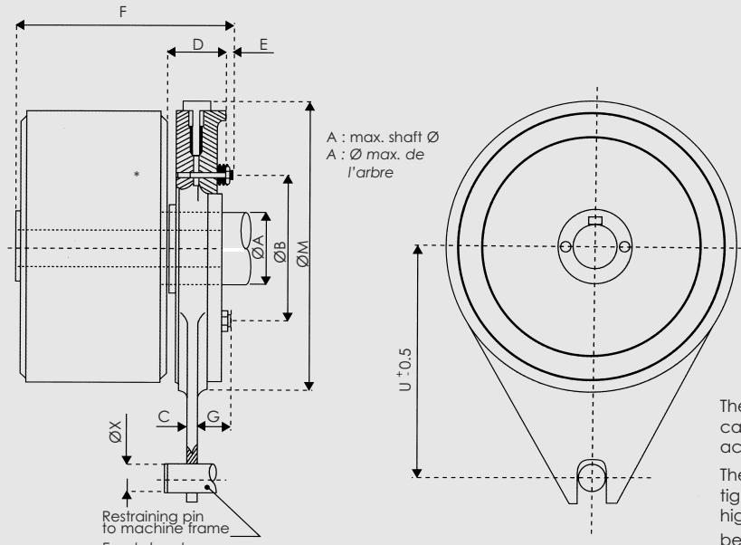
The REDEX friction torque limiter is based on a mono-disc design. Overload protection is obtained by slippage when loads exceeding the rated torque value. The use of the limiter is recommended when the driven machine is subject to frequent, and possibly dangerous, overloads.
