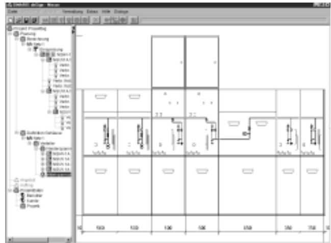
Illustration of the medium-voltage switchgear cabinet casing front view, including floor break-throughs
