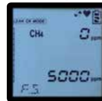
Leak Check Mode
