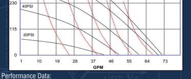
Performance curves are based on normal temperature (70°F), fresh water. The discharge volume and discharge head vary according to viscosity, specific gravity, etc. of the material to be transferred.
