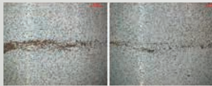
Fig. 36: Damage due to erosion in the running-in layer of a P1 plain bearing
