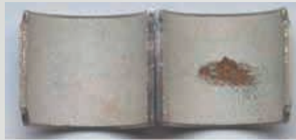
Fig. 35: Local damage caused by cavitation
