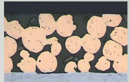
Fig. 5: Condition of sliding surface at end of the run-in
