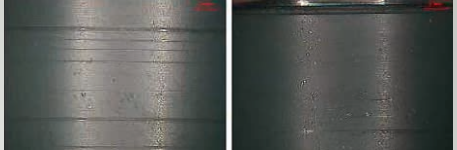
Fig. 37: P2 plain bearing, grooves in the sliding surface
